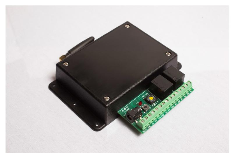
**POLD+** if you were to wire up a POLD sensor to the API (and it is polarized) the Sensor would have its black wire going to GND and its red wire going to POLD+. When the POLD+ goes to GND level, it trips.
